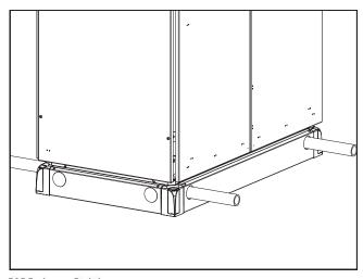
Ensure lifting rope angle is greater than 45° from horizontal
