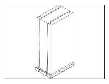
19-1-2 Ensure iLINQ is strapped or screwed to pallet before moving
